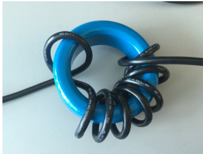
Figure 17. USB Cable Around Ferrite Bead
